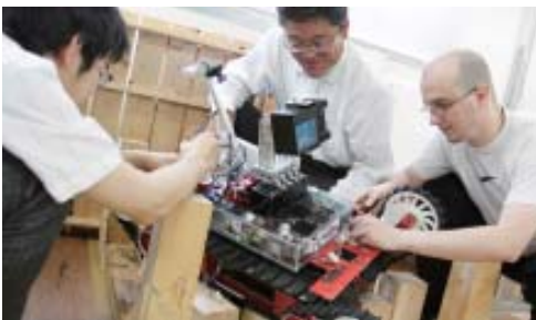
Kenaf (a tracked vehicle for exploration). This is remotely operated from a safe place by means of wireless LAN, and is capable of measuring 3D shapes.
